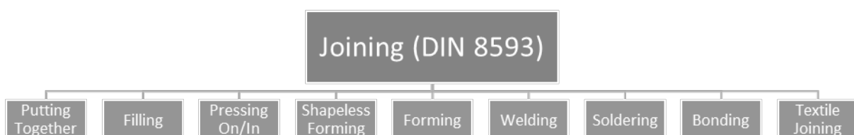
Figure 3. DIN Standard for Manufacturing Processes-Joining
