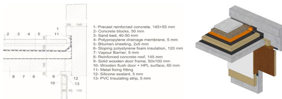
Figure 2. Renovation project of students' apartments at the Olympic Village, Munich 8 ; reproduced terrace detail in section and perspective
